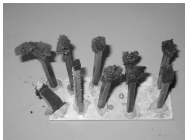
Figure 2 Photo of samples after oxygen index tests. Front row (from left to right)—samples 80, 81, 82, 84, 85. Back row—samples 89, 88, 87, 83, 86 (See Tables I and II for samples composition).
